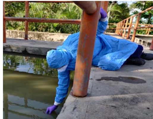
Collection of sewage sample from a sewage treatment plant in Hyderabad
